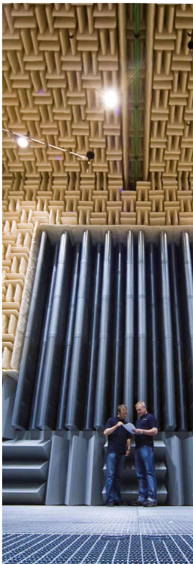
The world's most modern and largest test-bench for fans at the main location in Künzelsau (right)
