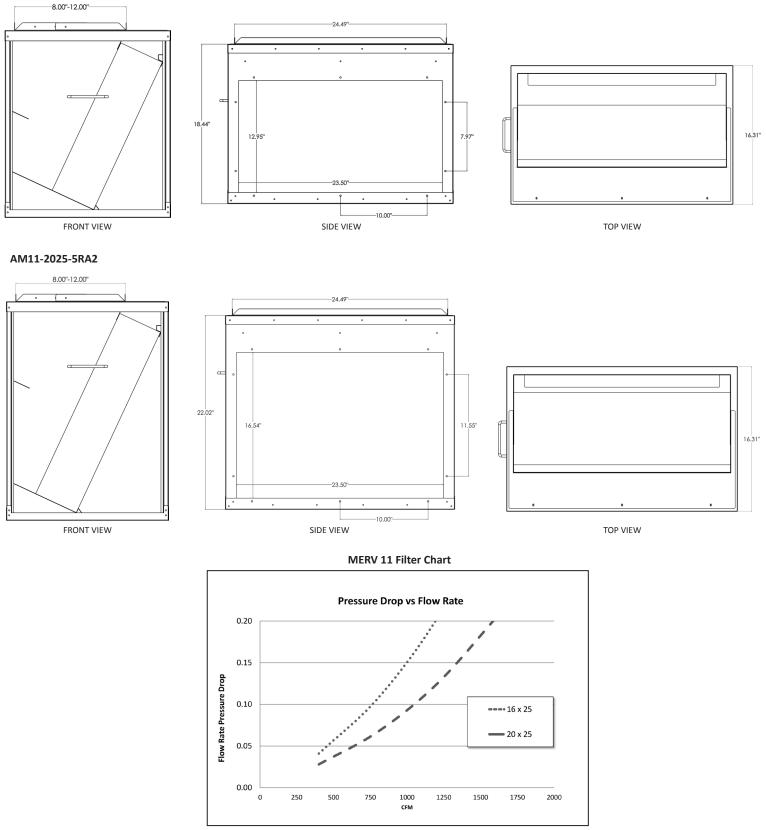
MERV 11 Filter shown, see filter specification sheet for MERV 13 pressure drop and flow rate information.
